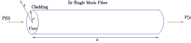
Figure 1. Parameter arrangement for the analysis of power in the modes in a length of amplifying fibre.
