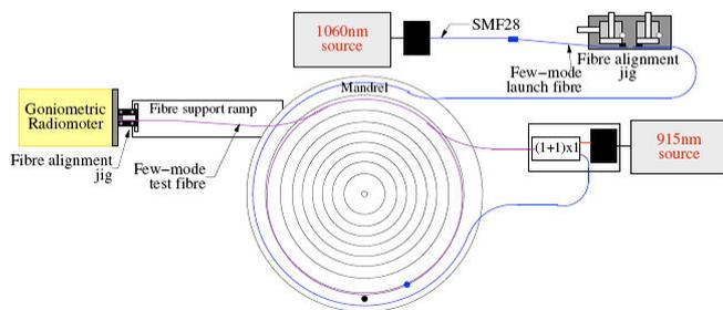
Figure 3. Layout of the system for a bend radius test of 2-mode fibre undergoing few-mode power amplification, showing up to the Goniometric Radiometer interface to the system.
