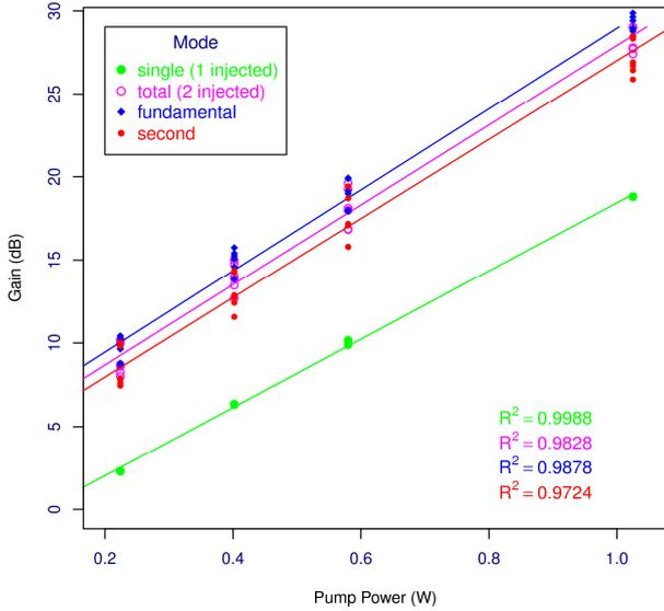
Figure 6. Ytterbium Doped Fibre Amplifier (YDFA) pump power to gain relationship for 1 and 2 injected modes.
