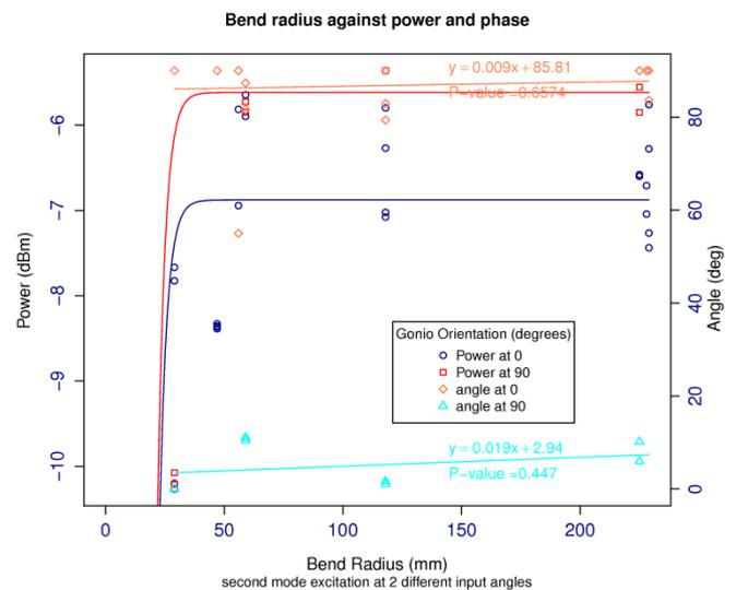
Figure 5. Bend radius tests for the unamplified fibre.
