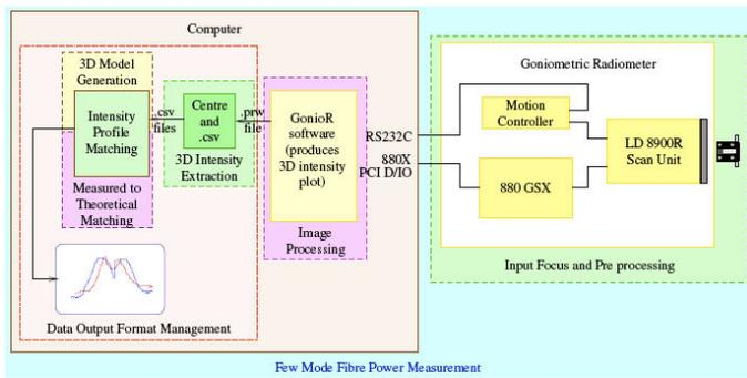
Figure 2. Total System Block Diagram, showing how hardware and software within hardware maps on to the functional decomposition.
